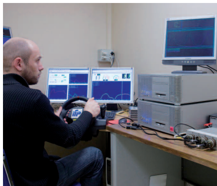
HIL simulation platform used for real-time testing of engine control systems.
