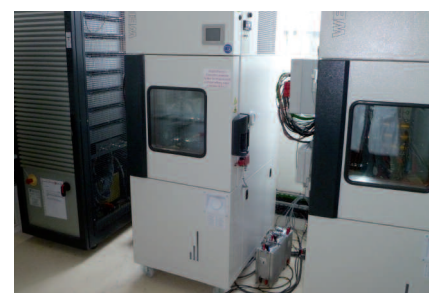
IFPEN's battery HIL bench is used to assess the behavior of a battery within an entirely virtual complex powertrain.
